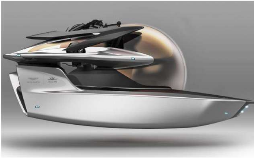
The three-person submersible can dive to 1,650 feet and hit speeds of 3.5 miles per hour. Source: Aston Martin
