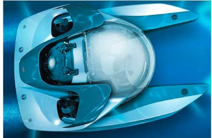
An acrylic bubble of a cabin maximizes underwater views. Source: Aston Martin
