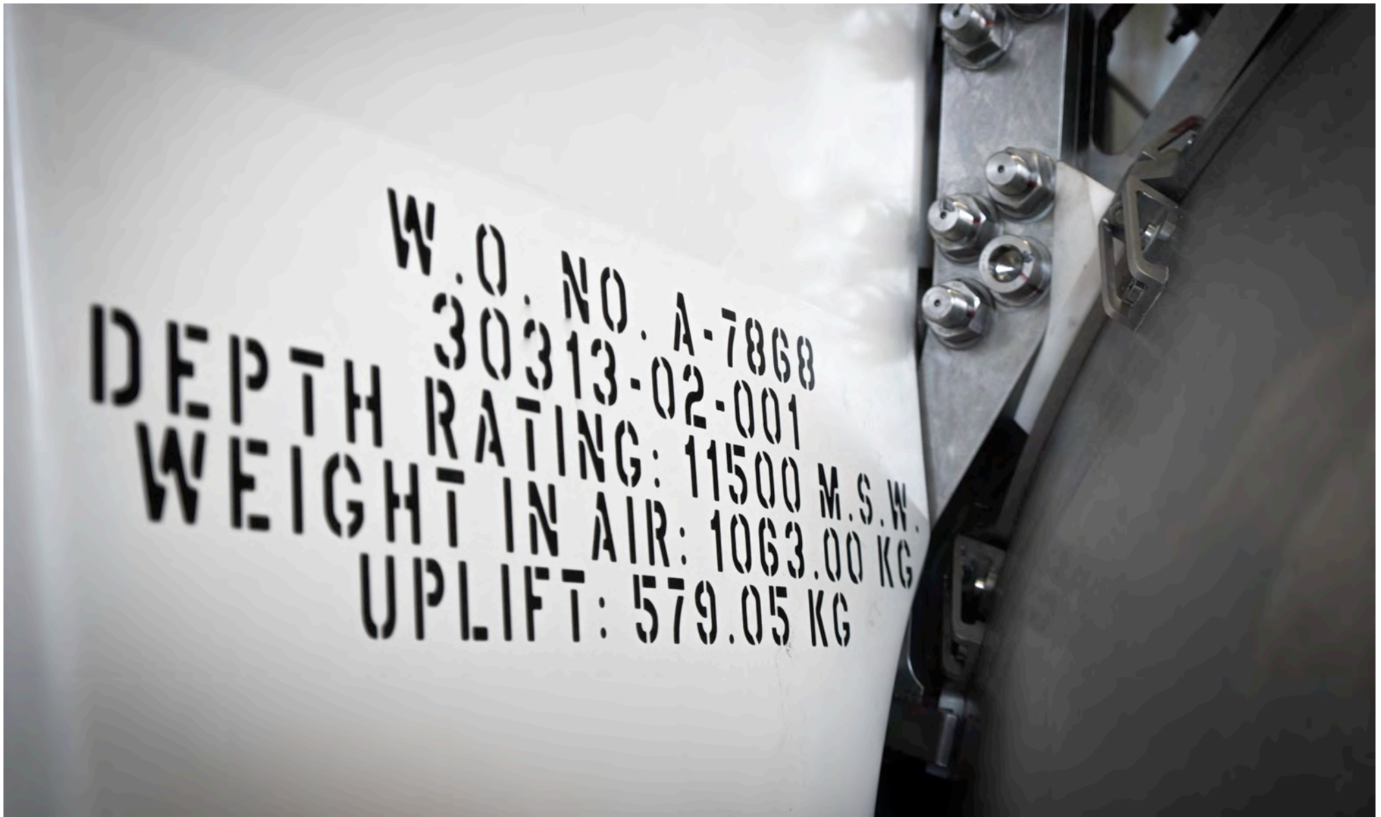
Full ocean depth pressure rated parts marked following QA acceptance, ready for assembly.
