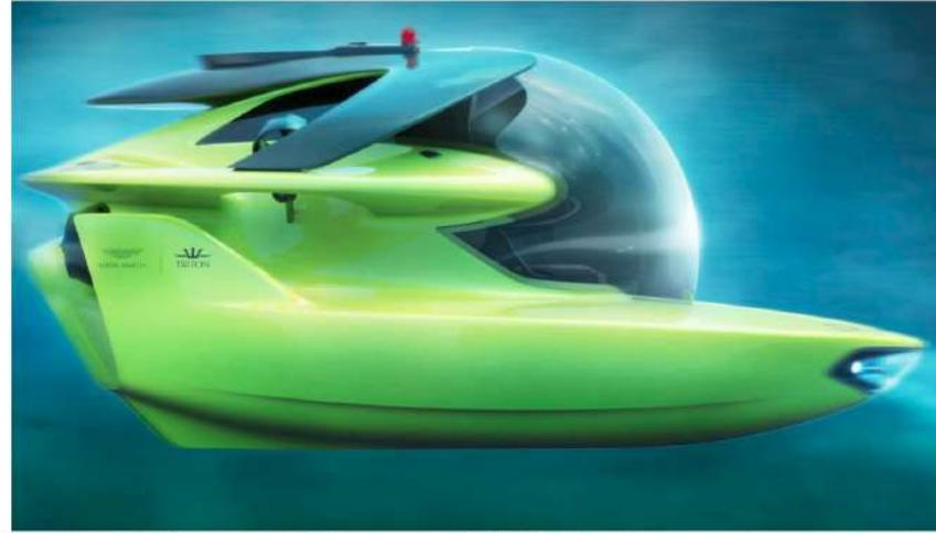
Not only is it a Bond villain's fantasy made flesh being able to achieve depths of 500m and reaching a sprint speed of 5 knots (and approximately four times the acceleration of Triton's current model), but it also boasts near 360 degree vision allowing passengers to soak up the alien sights of the deep sea.
