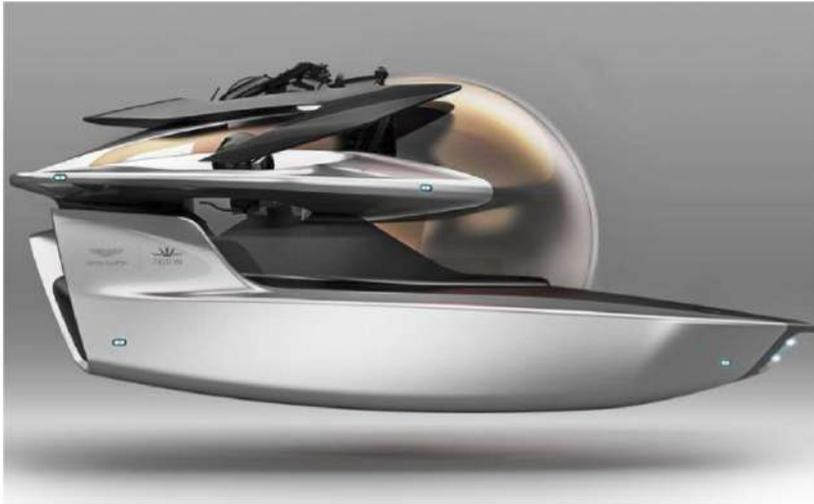
The three-person submersible can dive to 1,650 feet and hit speeds of 3.5 miles per hour. Source: Aston Martin
