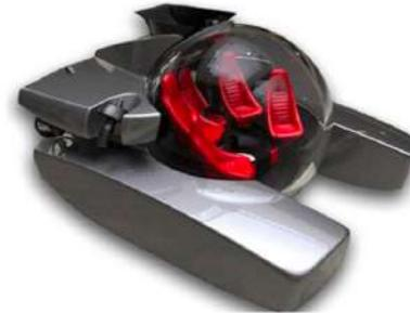
Described as "a salon under the sea," this 1650/7 Configurable promises to provide the ultimate experience in undersea opulence. This vessel will be able to dive to depths of 500m, though maintain an increased interior volume of a capacious 6.37 cubic metres and an interior design reminiscent of a yacht.
