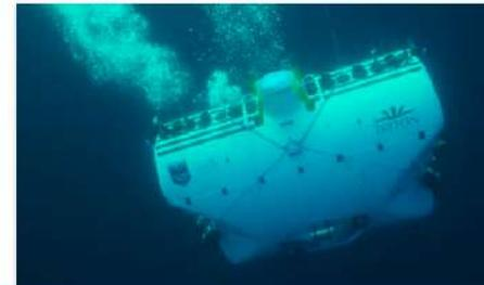
The 12-tonne submersible, with a top speed of roughly 1.5 metres per second, was launched from a dedicated support ship, the DSSV Pressure Drop. Limiting Factor represents a giant leap in Deep Sea exploration technology. It took 26 months to build after a year in the design phase.
