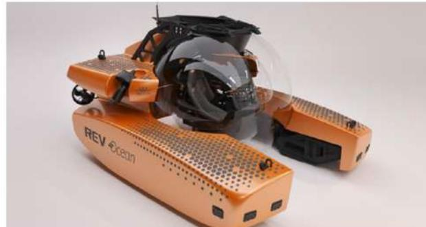
Assigned to Project REV, the world's largest explorer yacht-in-waiting, at the end of 2019, this remarkable submersible, which is currently under construction, is set to dive to an astonishing 2,286m, earning the title of the world's deepest diving acrylic pressure hulled submersible. It's a design set to push the technological and innovative standards of the industry while simultaneously allowing for a more comprehensive understanding of our oceans.
