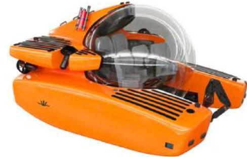
Featuring Triton's largest acrylic pressure hull produced to date, this six-person submarine was designed to deliver extraordinary experiences for larger parties of guests. Capable of reaching depths of 1,000m and boasting a staggered, stadium-seating arrangement, the 3300/6 offers a true shared experience exploring the world's oceans (and their floors).
